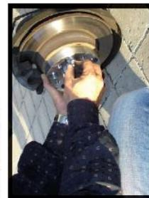
Mount the wheel spacer on the axle using the nuts/bolts which were included in the delivery. Tighten the nuts/bolts by hand.
